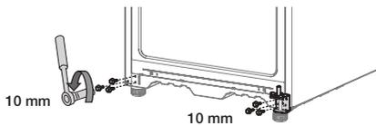
7. Separate the hinge shaft by using hex wrench first. Unscrew the bolt to remove the hinge riser and switch the side of the hinge shaft and the hinge riser.
