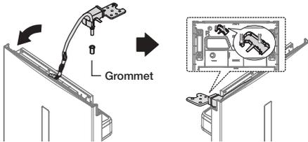
14. After switching the hinge, close it with the wire cover on the top of refrigerator door.
