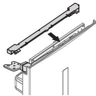
15. Take off the handle cover and remove the screws, make sure to detach the caps and the handle from the left to right side of the door. (Make sure to cover the left side with detached caps.)
