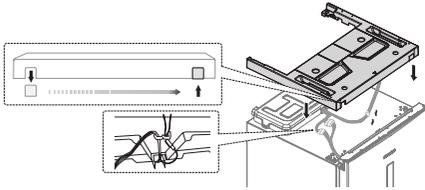
19. Tighten 4 screws back to its place.
