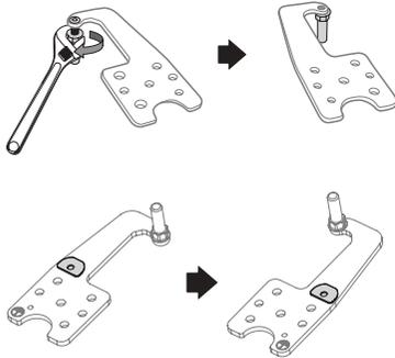
13. Reassemble the hinge on the refrigerator door by reversing the step 11. Make sure to use left side hinge cover (which can be found underneath the removed plastic cover from step 2) and remove the grommet. After reassembling the hinge, wire and the hinge cover, switch the side from right to the left.
