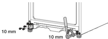
9. Remove the screws on the bottom left and right side of the refrigerator door. Switch the side of the door stopper from right to the left. Hinge riser should be switched as well.
