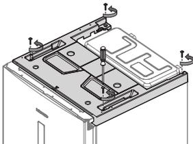
2. Remove the plastic cover and make sure to disconnect the wire connected to it. After removing the plastic cover, check the parts for reversing the door.
