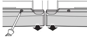
3. Remove the screw from the each of the product and attach them back after putting the bottom fixer.
