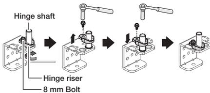
8. Attach the hinge on the bottom left side of the refrigerator where bolts were previously removed in step 6. Screw the bolts that were removed on the bottom right side of the refrigerator for the future usage. Switch the the Leg from the left to right.
