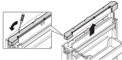
11. Remove the hinge and the grommet from the refrigerator door. Detach the right side hinge cover and pull the wires out of the hinge cover.
