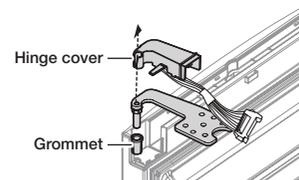
**CAUTION** Be careful not to damage the electrical wires when removing the hinge cover.
