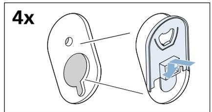
5. Press the cover cap down firmly at the top, while at the same time pushing it downwards until you hear the hooks clicking into place.
