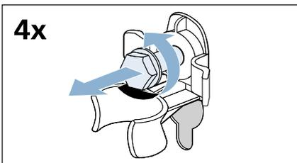
3. Remove the sleeves. Remove the mains cable from the holders.
