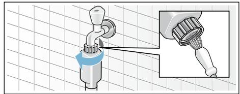
6. For standard and Aqua-Secure models, clean the filter on the rear of the appliance: Remove the hose from the rear of the appliance. Use pliers to remove the filter and then clean it.
