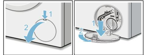
4. Take the drain hose out of the retainer. Remove the sealing cap, allow the detergent solution to flow out into a suitable container. Replace the sealing cap and place the drainage hose in the retainer.
