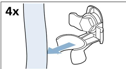
2. Use a WAF13 spanner to undo and remove all four transport lock bolts.
