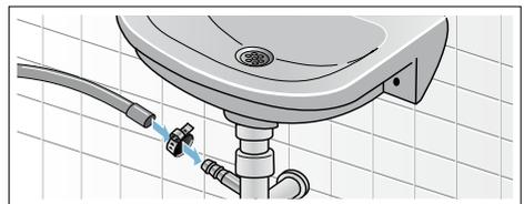
■ **Outlet into a plastic pipe with rubber bushing or into a drainage pit**
