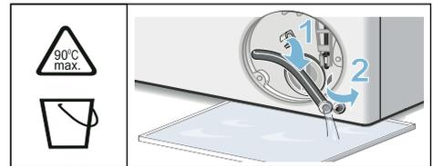
5. Carefully unscrew the pump cover, residual water may leak out. Clean the interior, pump cover thread and pump housing. The
