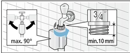
**Note:** Open the water tap carefully, checking the leak tightness of the connection points. The screw connection is under mains water pressure.
